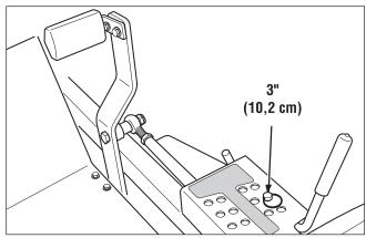
Figure 38. Deck Lift Pedal & Pin Position
